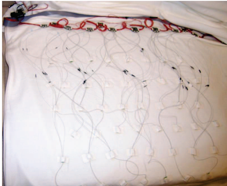
Figure 2: View inside the Touch Blanket, showing the wiring and part of the matrix of vibration motors. The motors are attached to the fabric with white adhesive tape.
