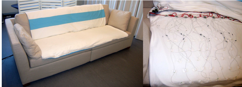
Figure 1: (left) Touch Blanket spread over a sofa; (right) inside view, showing the wiring and part of the matrix of vibration motors attached to the fabric.
